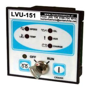
If a fault condition occurs, the FUEL solenoid will be deenergized. If the 'Energize to Stop' option is selected, the AUXILIARY relay output will be energized during stop timeout and the led associated with this condition will turn on.
